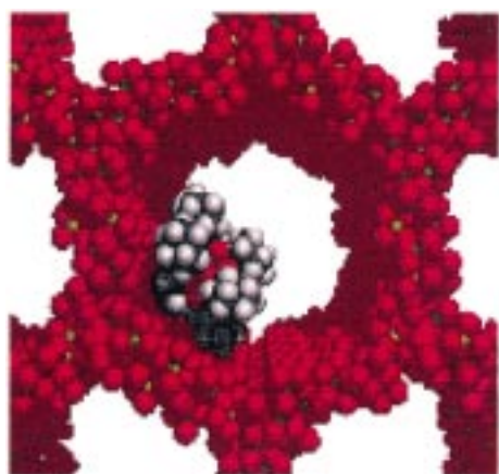
Figure 1. Graphical representation of the adsorption of 9 in the \approx 30 Å pores of all-silica MCM-41.
